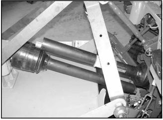
Figure 3. Drive Halves Placed Parallel
